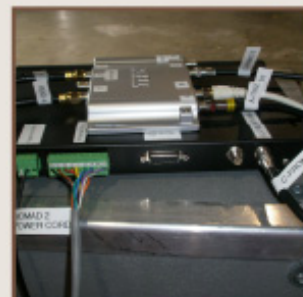
Back view of the Nomad 2 and side view of the TERK. Coax cables are connecting the Nomad 2 to the televisions.
