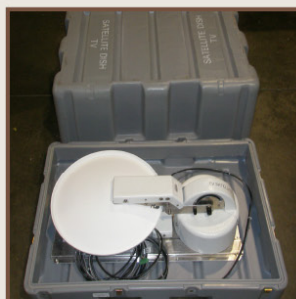
The satellite case opened with the satellite in the stow position.
